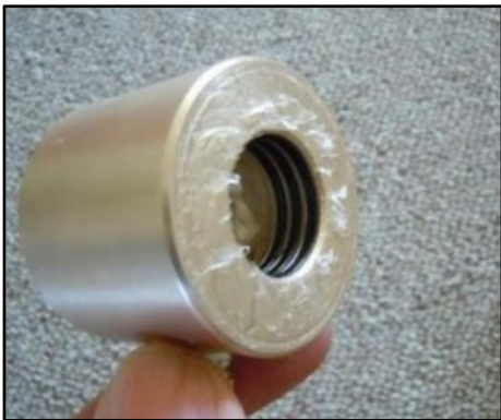
quad rings in water swivel
