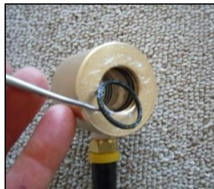
quad ring removal with dental tool
