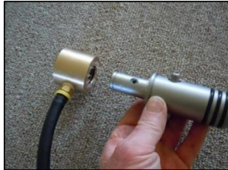
dis-assembled water swivel
