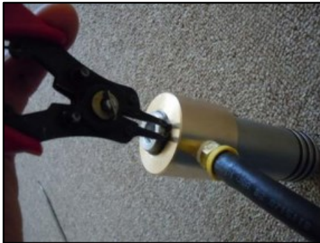
dis-assembled water swivel
